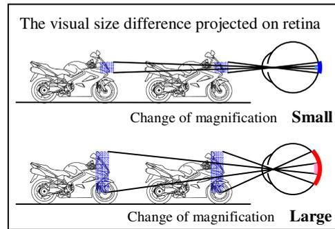
**Figure 3. Principle of enhancing a sense of speed**
