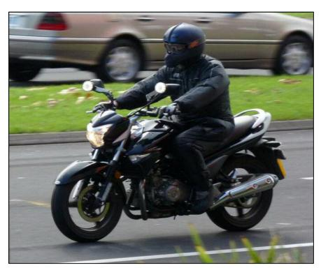
Figure 10: Trials motorcycle, displaying upper DRLs ('V' configuration) with rider wearing black clothing and helmet cover
