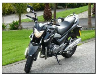
Figure 8: Trial motorcycle, displaying both pairs of Daytime Running Lights (DRLs, in this case the Y' configuration)
