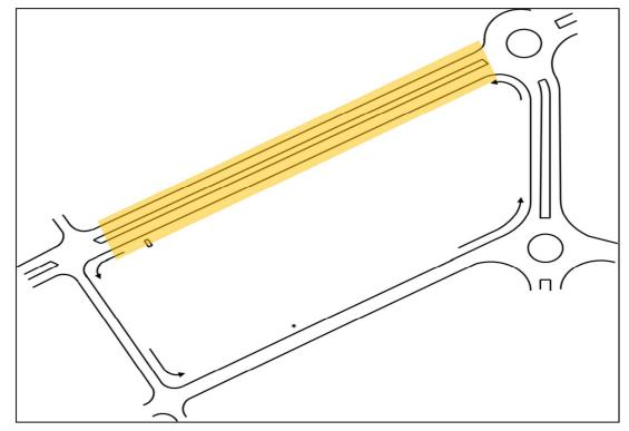
Figure 11: Plan view of trial circuit (not to scale). Small rectangle to left is approximate observation vehicle location. Arrows indicate direction of travel around circuit for motorcycle. Asterisk marks waiting position for motorcycle. Shaded section expanded in Figure 12
