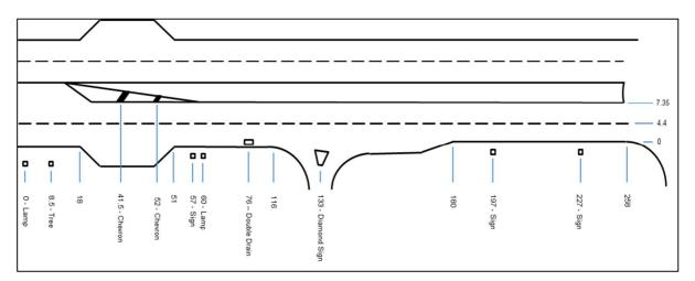
Figure 12: Close up detail of approach road with distances from lamp on left (0) in metres (not to scale). Observation vehicle was parked roughly half way between lamp (0) and tree on left in single-car setup. Second car was parked just to left of lamp (0) in two-car setup
