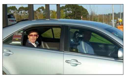
Figure 3: 'Participant' (MP) seated in rear of trials car, with video camera attached to driver's side window and experimenter (SH) in front passenger seat. Note 'view obstructer' attached to rear quarter-light window
