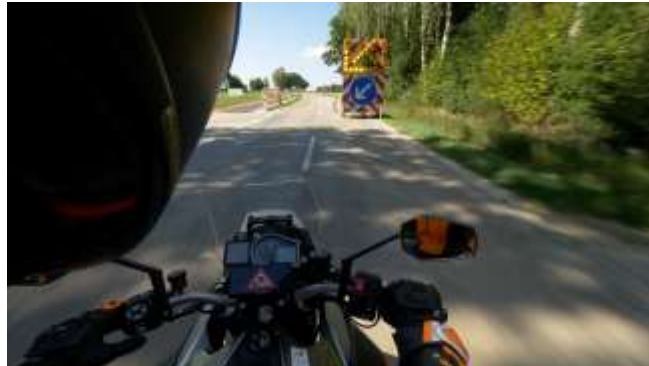
The motorcycle rider gets a information on the HMI about a possible conflict with another vehicle when overtaking
