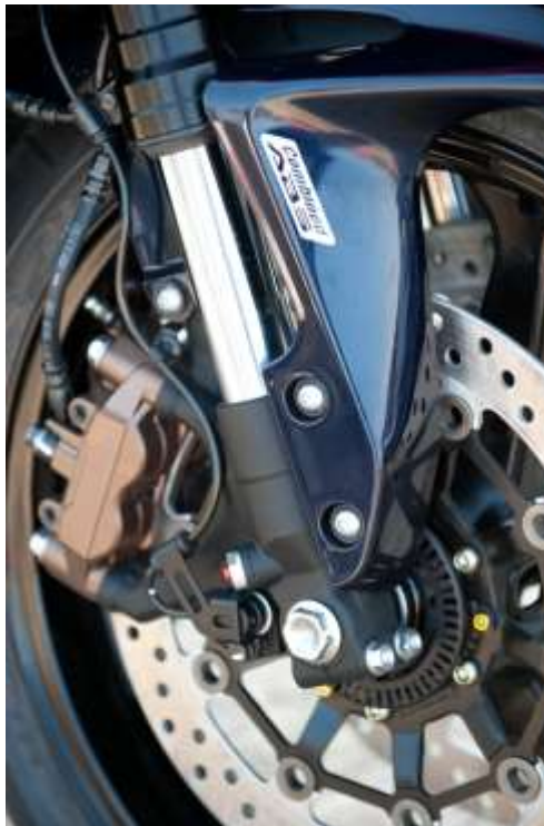
Front wheel disk brake fitted with ABS
