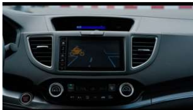
Connectivity allows informing a car driver of an oncoming motorcycle
