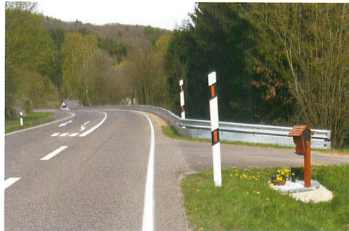
➤ After: A staging point for a left turn; visibility of the junction enhanced with supersize guidance posts.
