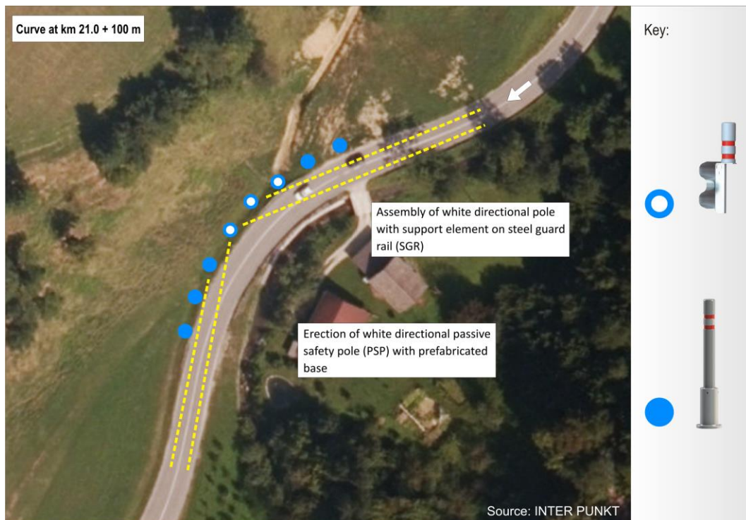
Figure 32: Example of determining the locations of white directional passive safety poles (PSP) with prefabricated bases, and of white directional poles with support elements for assembly on steel guard rail (Source: INTER PUNKT d.o.o.).
