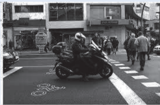
Figure 8.2. Advanced stop line in Madrid
