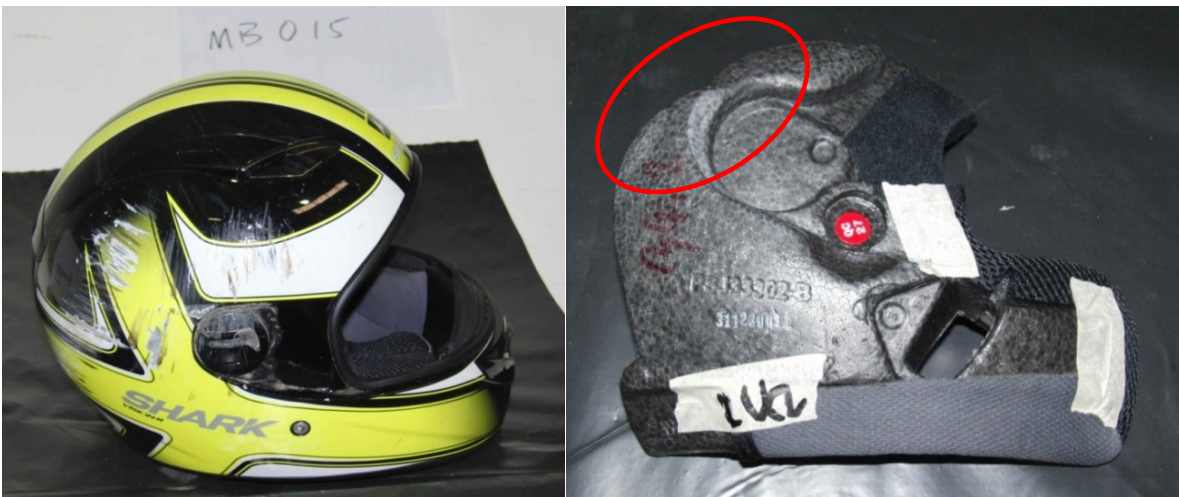
Figure 51: External damage and corresponding damage to the internal protective liner of the helmet
