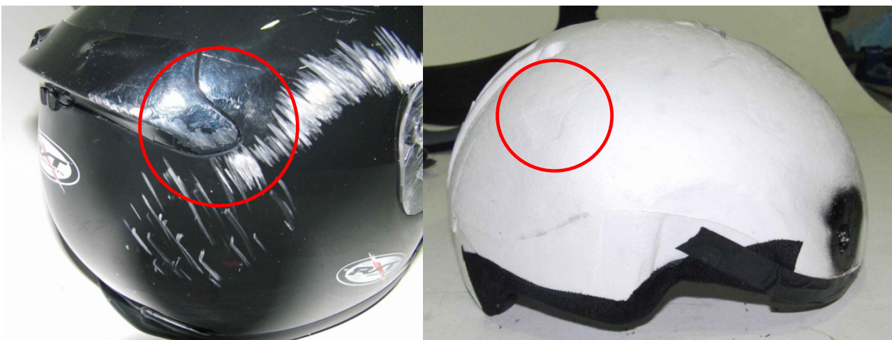
Figure 51: External damage and corresponding damage to the internal protective liner of the helmet
